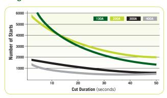
Note: The capabilities shown in this table were obtained by using new consumables, correct gas and current settings, accurate torch height control and with the torch perpendicular to the workpiece. Parts life shown for 130A and 200A are non bevel parts. Please contact Thermal Dynamics for more information.
