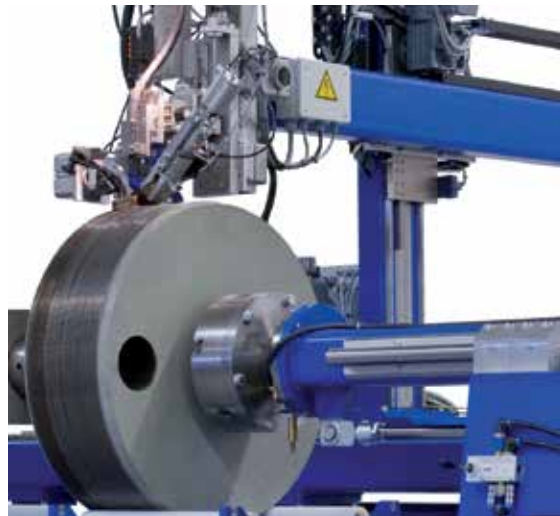
Automated welding head
