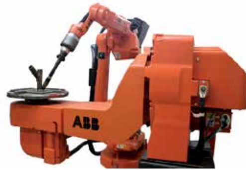
Robot welding cell for MAG welding with 2 axes positioner and torch cleaning station
